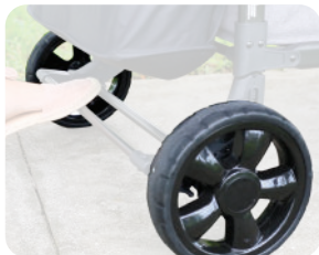
All-Terrain EVA Tyres with Bearings & Suspensions
